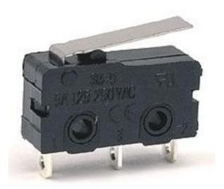
You'll note that there are three contacts here, one is the signal and the other two are for the normally closed and normally open contacts. By "normally closed," we mean that this contact is connected to the signal when the switch is NOT depressed, and normally open means this contact is only connected to the signal when the switch is depressed. The only two contacts we'll use are the normally open and the signal.
