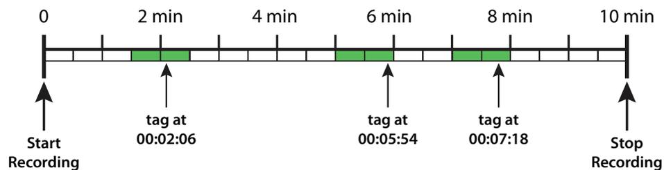
Using the Loop recording method, recording starts when the **REC** button is pressed, but the captured video isn't saved until **Tag** is pressed. When **Tag** is pressed at 00:02:06, a short clip, called a **loop**, is saved, as indicated by the short green segment at that point. When **Tag** is pressed at 00:05:54, another loop is saved, and finally, when **Tag** is pressed at 00:07:18, another loop is saved.
