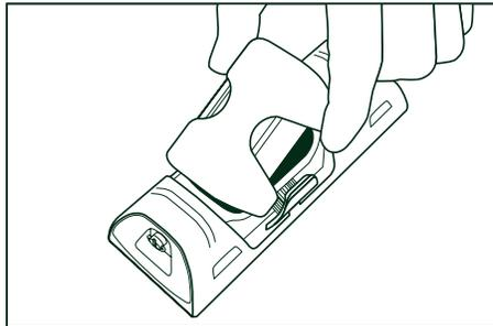
2. Remove the Input/Output cover from the bottom of the recorder, and install the SD card included with the POV.HD.
