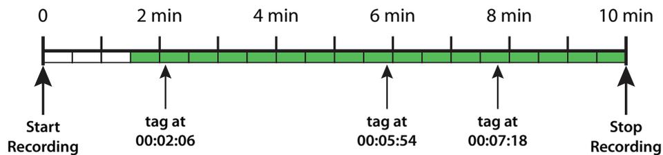
In effect, Loop & Forward allows you to record using the Clip method, without starting the clip until the action starts. You can get everything set up, stow the recorder, and get yourself over to the starting line without the need to record fifteen minutes of waiting time which you're going to want to edit out later anyway. When the gun's about to sound, hit the tag key on the remote and real recording starts.
