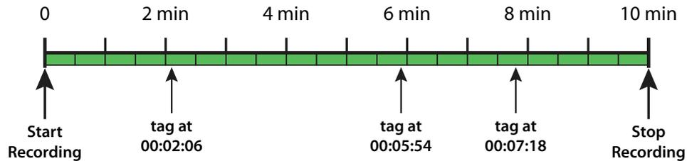
Using the Clip recording method, recording starts when **REC** is pressed and runs continuously until **REC** is pressed again. This is exactly the way a standard video recorder works. In addition, each time the **Tag** key is pressed, a **tag** is recorded, for later possible use with the built-in editing features.
