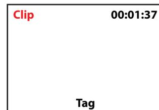
3. To tag the clip being recorded, press the **Tag** soft key.
